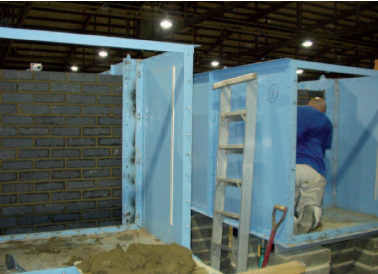
Figure 7.4 Constructing wall test panels in the laboratory test rigs
