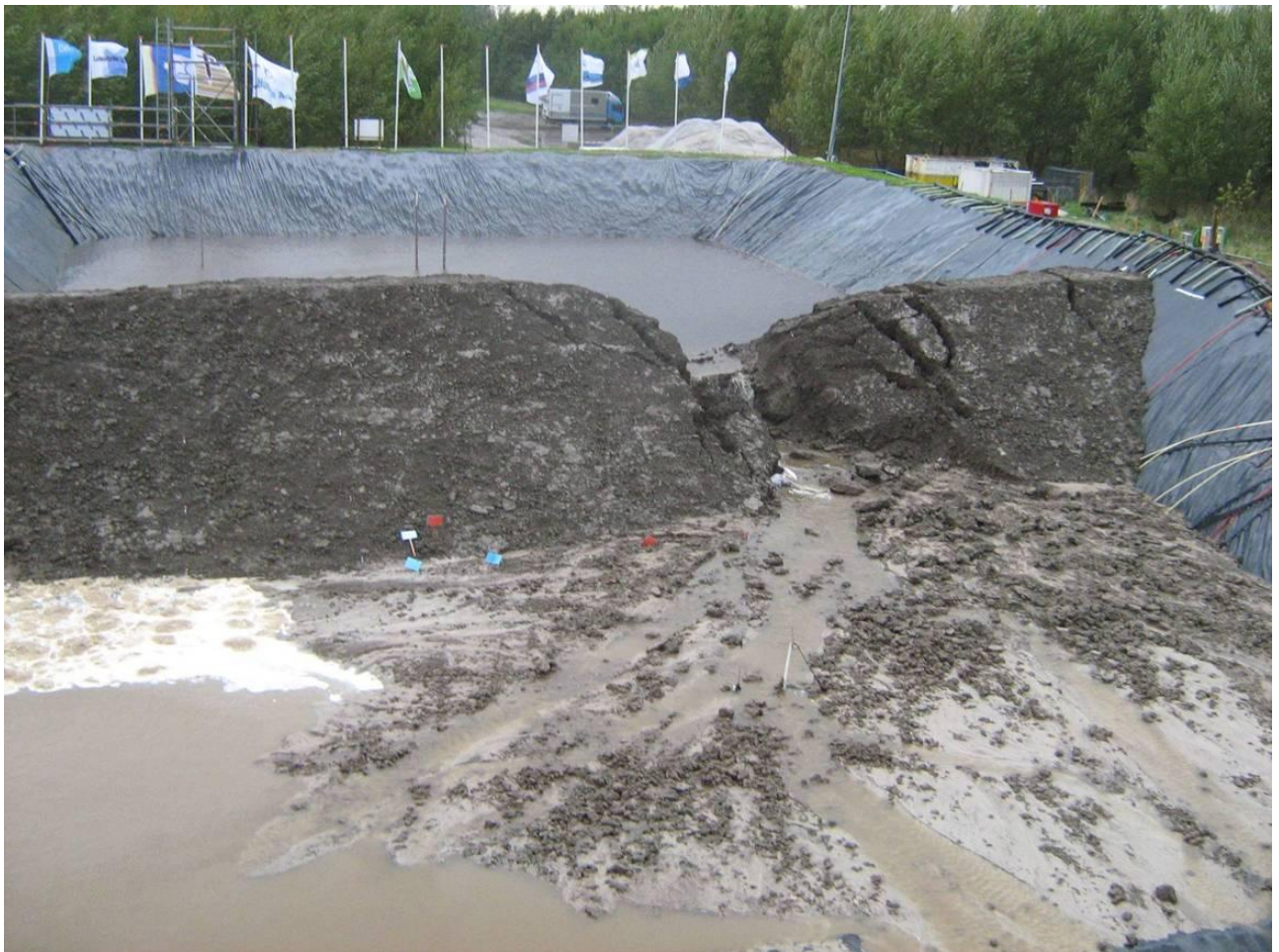
Figure 3.3 Failure due to backwards erosion; piping test at Ijkdijk, The Netherlands
