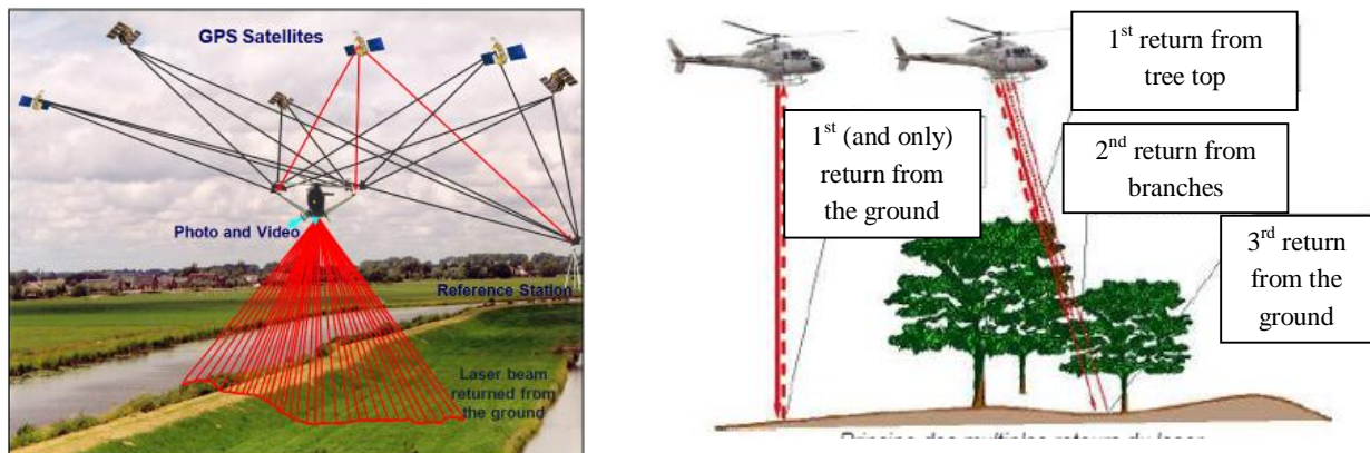
Figure 3.11 Lidar acquisition (left) and multiple return (right) principle
