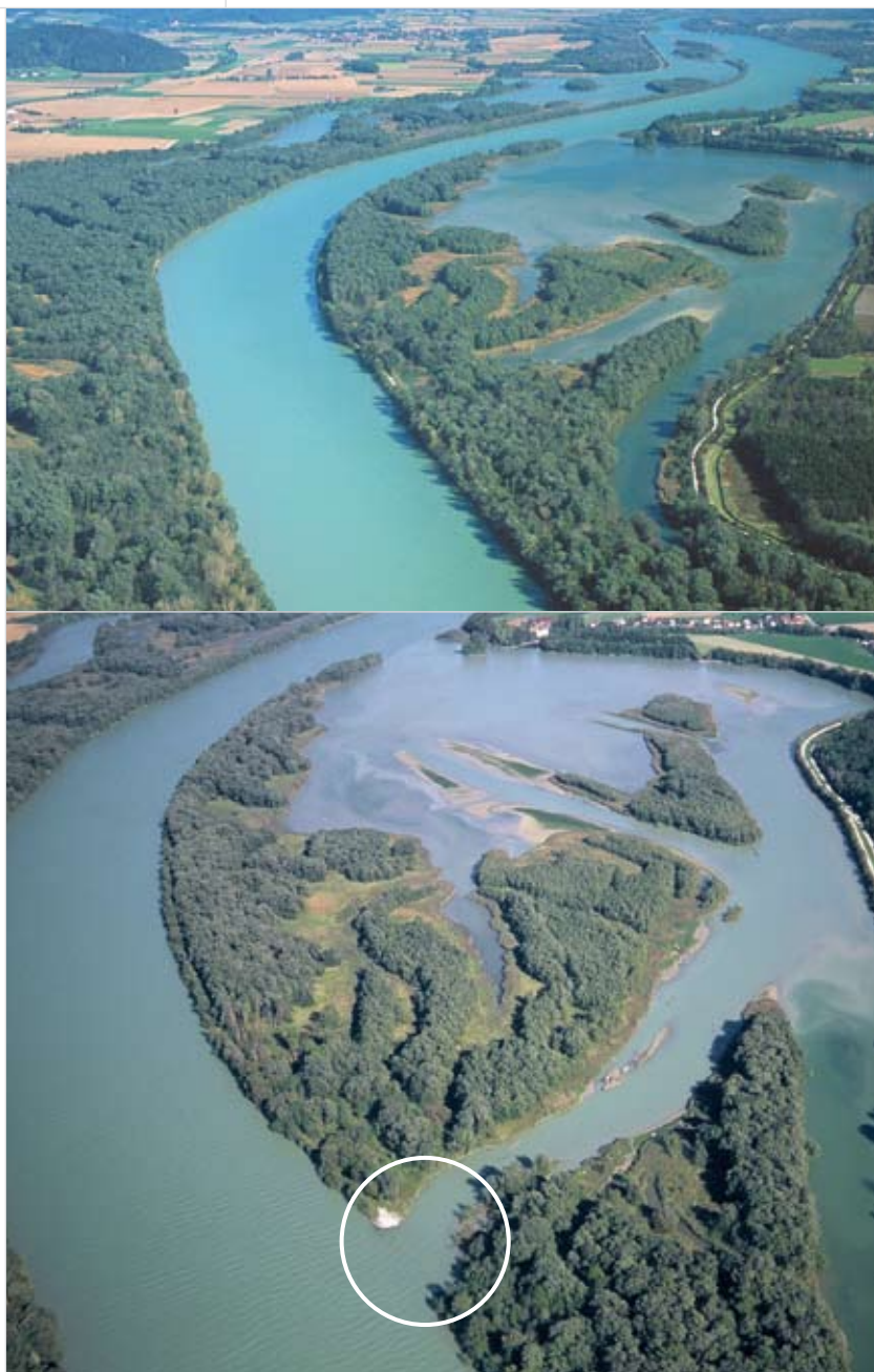
River Inn embankment opening – before the project work (top) and after (below)
