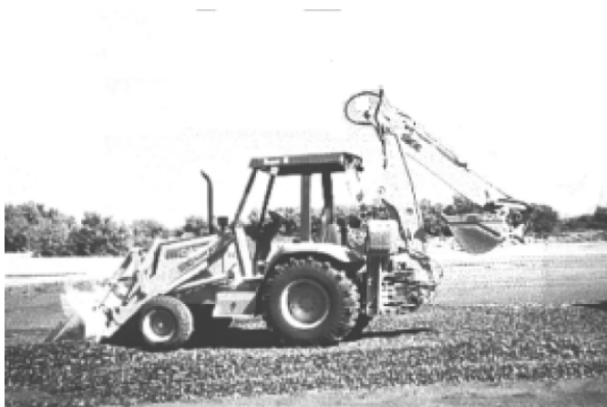
Figure 7-9. Backhoe mounted on farm tractor.
