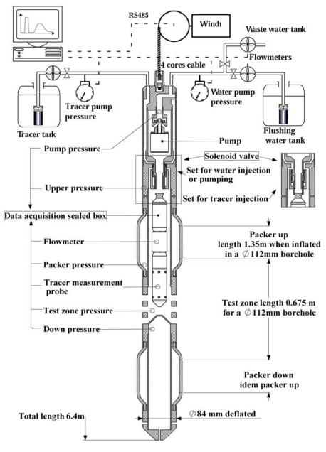
Figure 8. Schematic of the downhole probe and the surface equipment.
