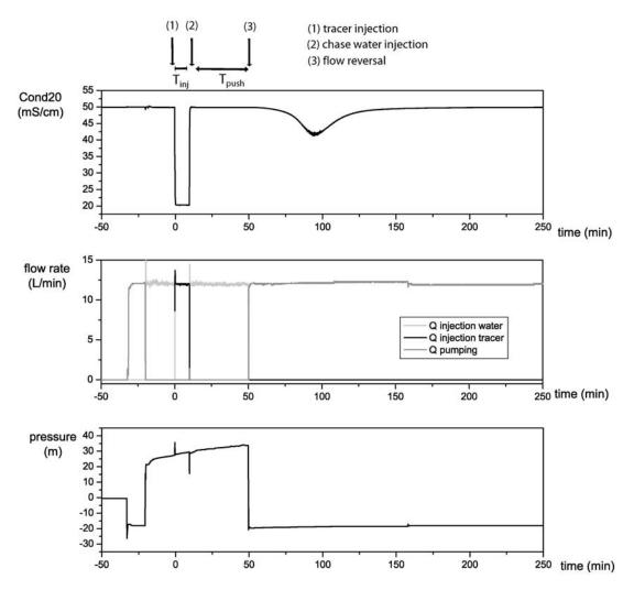
**Figure 7.** Example of SWIWT monitoring (tracer test 1–1). Evolution of (top) conductivity, (middle) flow rates, and (bottom) pressure as a function of time. The experiment was performed at 94 m depth. The tracer injection time is  $T_{inj} = 600$  s and the flushing water injection duration is  $T_{push} = 2400$  s. The flow rate is  $2 \times 10^{-4}$  m<sup>3</sup> s<sup>-1</sup> (i.e., 12 L min<sup>-1</sup>). The resident water conductivity is approximately 50 mS/cm.
