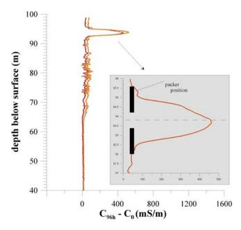
**Figure 9.** Difference between induction log in natural conditions ( $C_0$ ) and induction log 96 h after the injection of 3 m<sup>3</sup> of freshwater between packers at 94 m in well MC2. The difference is shown as a function of depth for both the short- and long-range induction logs. The positive anomaly at 94 m marks out the location of the injected plume of freshwater 96 h after injection.
