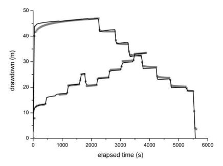
**Figure 5.** Step drawdown test results in the interval 93.55–94.35 m, with flow rates ranging between 1.113 m<sup>3</sup> s<sup>-1</sup> and 3.073 m<sup>3</sup>. Dotted curves are measured data and continuous curves are outputs from the fitted model (transmissivity =  $1.6 \text{ m}^2 \text{ s}^{-1}$ ).
