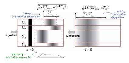
**Figure 1.** Schematic representation of the reversible-irreversible dispersion. SWIW tracer tests act to cancel long-range velocity correlations. Gray zones denote the concentration distribution (left) at the end of the push duration ( $t = T_{push} + 1/2 T_{inj}$ ) and (right) when the tracer mass center is back to the initial position at time  $t = 2T_{push} + T_{inj}$ . The black zone on the left corresponds to the tracer at the initial time (t = 0).
