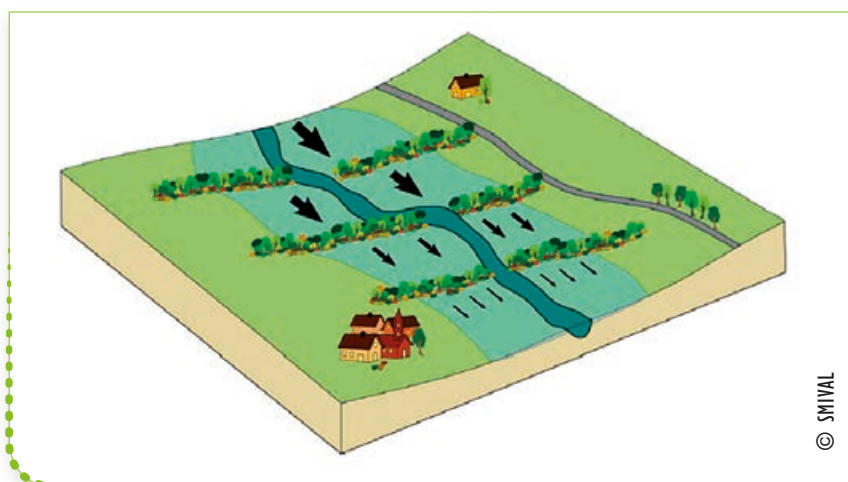
Floodbreaking hedges obstructing the flow and slowing down running water
