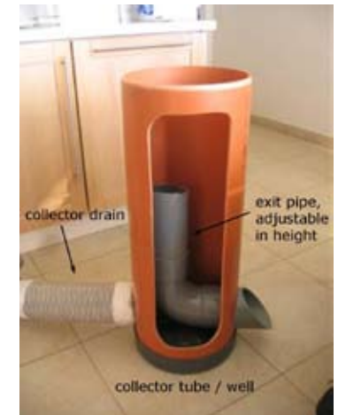
Figure 2: Collector tube well
