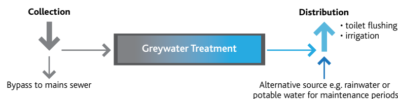
Figure 6. Schematic of greywater reuse system
