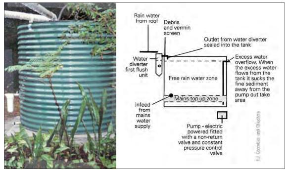
Figure 1. Rainwater tank components. (Coombes and Kuzcera 2001.)
