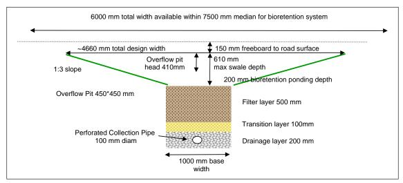
Figure 10. The completed bioretention system design for the worked example.
