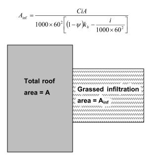
Figure 6. Example definition of a catchment area where the infiltration surface is located external to the defined site area.
