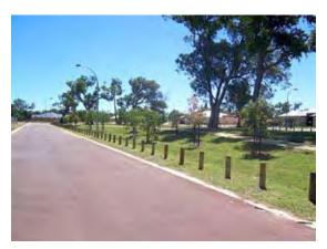
Figure 3. Bollards used to prevent vehicular access onto a swale for conveying road runoff in Mandurah. (Photograph: Grahame Heal, City of Mandurah.)
