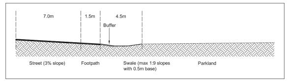
Figure 8. Cross section of proposed buffer/swale system.
