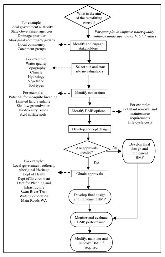
Figure 5. Flow chart showing the simplified design process for retrofitting projects.
