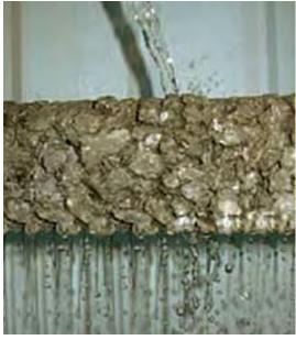
Infiltration through pervious paving. (Source: Washington Aggregates & Concrete Association 2006.)
