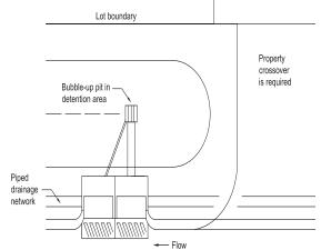
*Figure 4. Plan view of the pipe network with bubbleup connection to the piped system. (Source: TME 2003.)*
