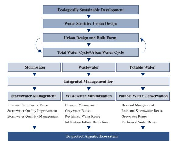
Figure 6: Interactions between ESD, WSUD and the Urban Water Cycle (Institution of Engineers, 2003)
