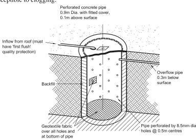
Figure 3. Leaky well infiltration system.
