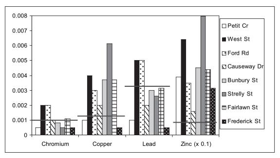
Figure 20. Average heavy metal concentrations found in Busselton stormwater drains in 2002-03. Lines indicate guidelines for protection of aquatic ecosystems (ANZECC and ARMCANZ, 2000).
