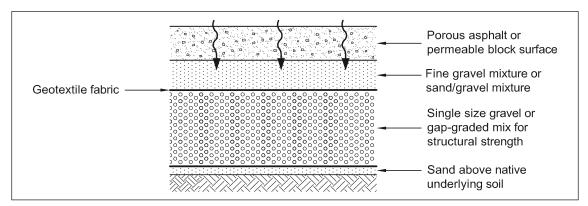
Figure 3. Schematic of a section through pervious pavement.
