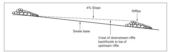
Figure 4. Location of riffles in a swale.
