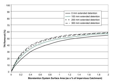
Figure 5. Bioretention system TN removal performance.
