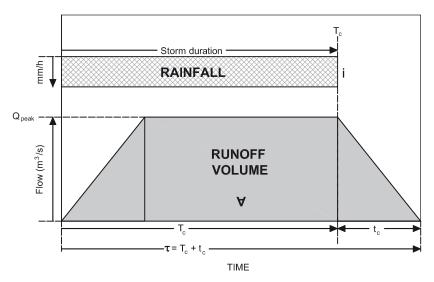
Figure 3. Simplified inflow hydrograph (for use in design without hydrologic modelling).
