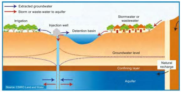
Figure 1. Conceptual Model of Aquifer Storage and Recovery Bore. (Source: CSIRO 2000.)
