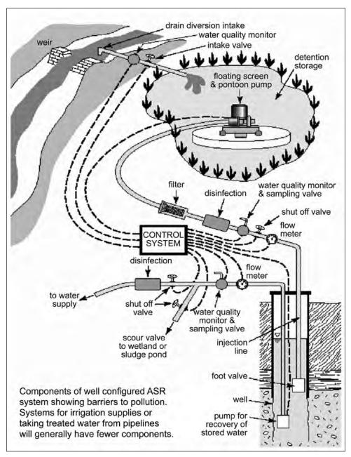
*Figure 2. Components of a well-configured MAR system. (Source: adapted from Department of Water, Land and Biodiversity Conservation, undated.)*
