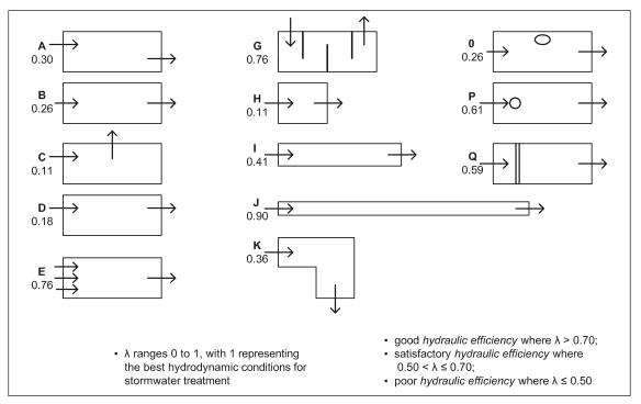
Figure 3. Hydraulic Efficiency ( $\lambda$ ) is a quantitative measure of flow hydrodynamic conditions in constructed wetlands and basins.  $\lambda$  ranges from 0 to 1, with 1 representing the best hydrodynamic conditions for stormwater treatment. (Source: Engineers Australia 2006.)
