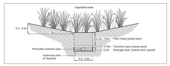
Figure 6. Typical liner arrangement for an impervious bioretention system.
