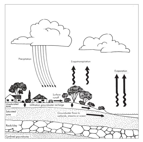
Figure 1: The hydrological cycle
