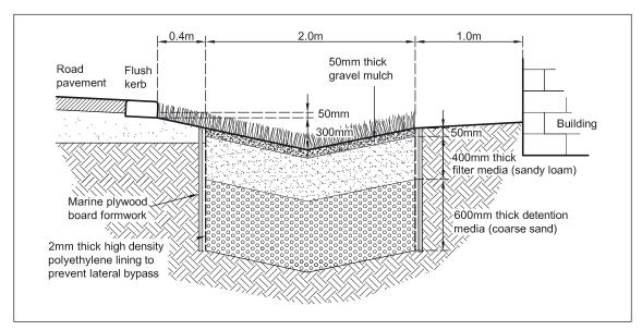
Figure 7. Typical liner arrangement for a pervious bioretention system.
