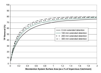
Figure 4. Bioretention system TP removal performance.
