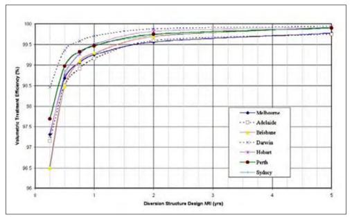
Figure 3. Treatment efficiency for various design ARIs. (Source: Wong et al. 1999.)
