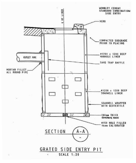
Figure 16. Standard combination gully / soakwell.
