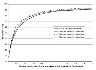
Figure 3. Bioretention system TSS removal performance.
