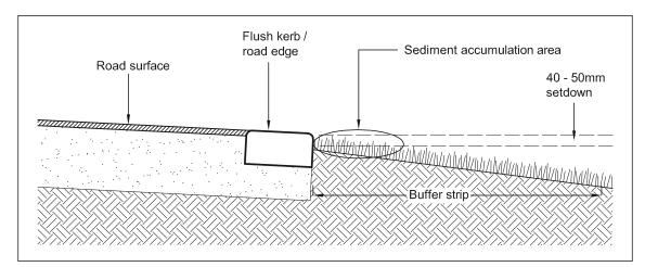
Figure 6. Edge setdown details for buffer strips.
