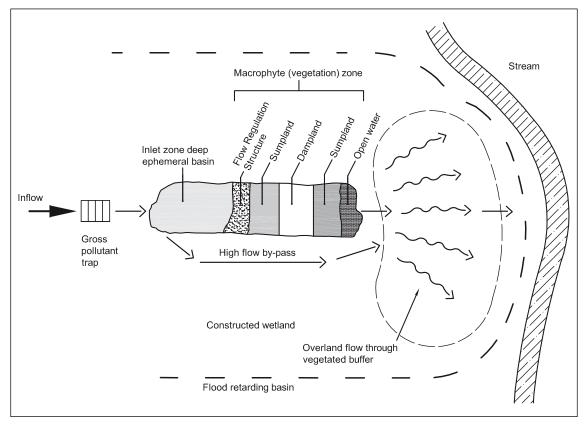
Figure 4. Bathymetry of a constructed wetland.
