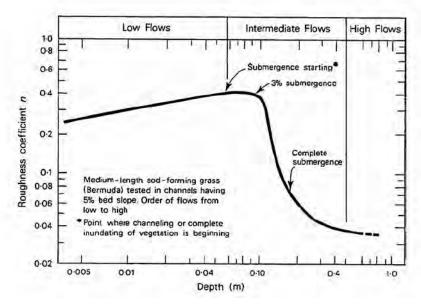
Figure 5. Impact of flow depth on hydraulic roughness. (Source: Engineers Australia 2006.)
