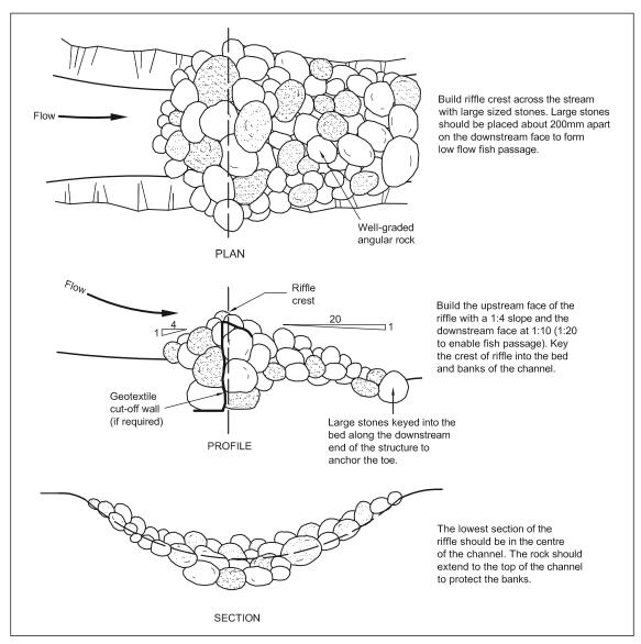
Figure 7. Design details for riffle construction.
