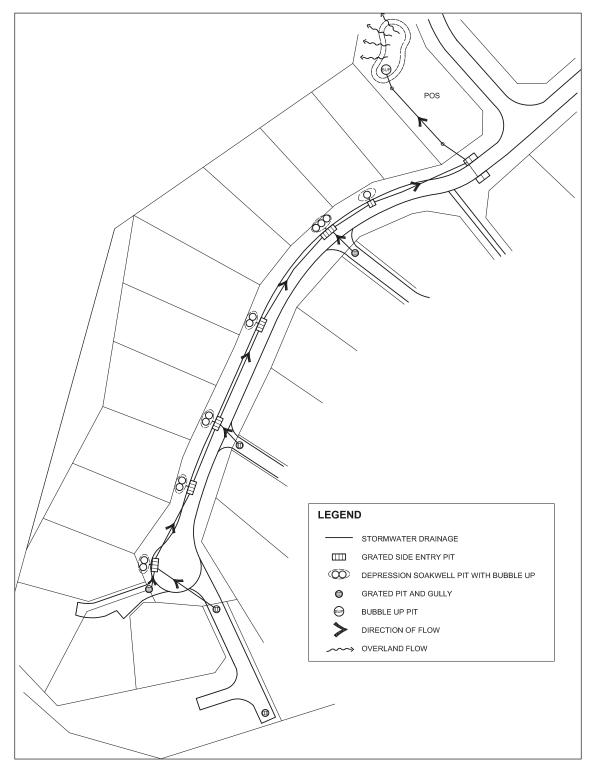
Figure 2. Boronia Ridge drainage plan. (Source: Department of Water.)
