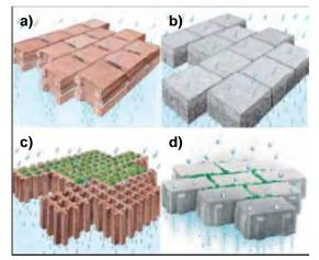
Figure 2. Types of permeable paving: a) pavers with canals b) porous pavers c) greened permeable pavers with small apertures d) greened permeable pavers with wide joints. (Dierkes et al. 2002.)
