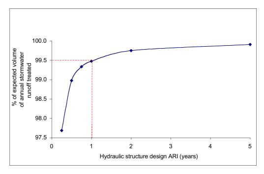
Figure 1. Treatment efficiency of stormwater hydraulic structures for Perth, Western Australia (adapted from Wong, 1999)
