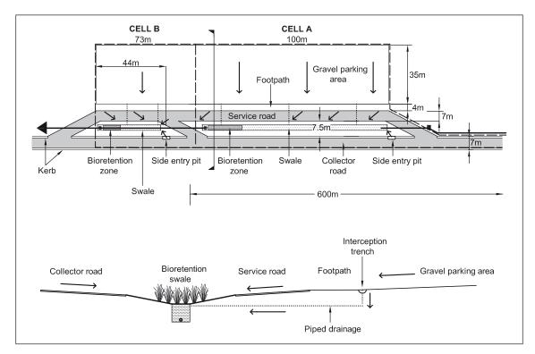
Figure 8. Catchment area layout and section for worked example.
