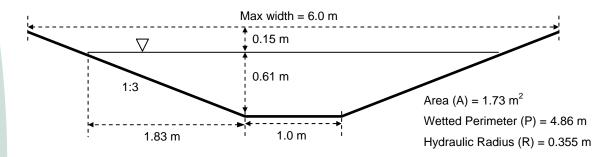
Figure 9. Swale dimensions for the worked example.
