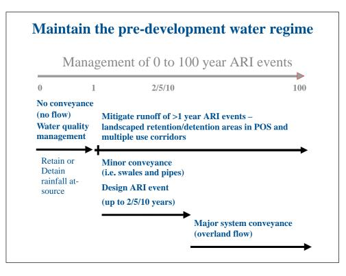
Figure 2. Approach to maintaining pre-development hydrology.
