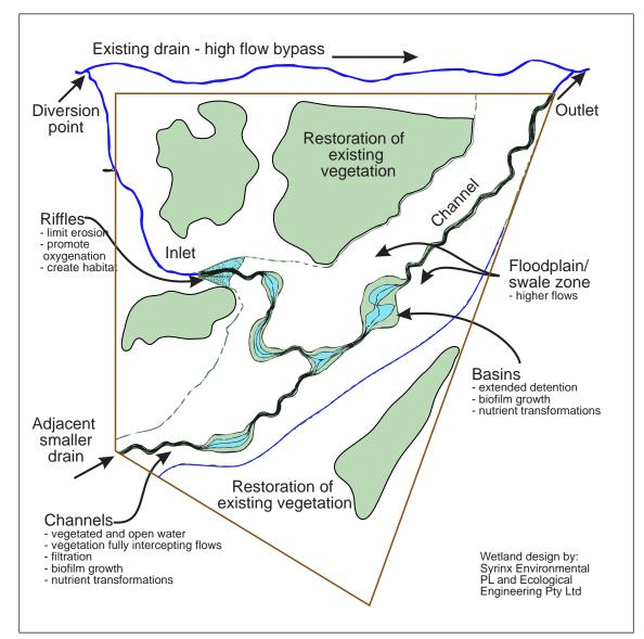
*Figure 5. Example of a constructed wetland design, showing key components of an ephemeral wetland.* (*Department of Water & Swan River Trust, in preparation.*)
