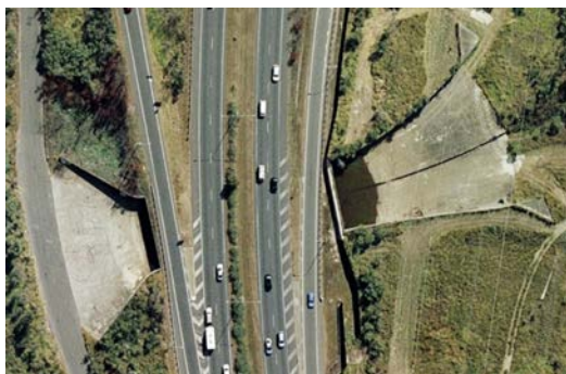
Figure 9.12 – Minimum energy loss culvert on Gateway Motorway
