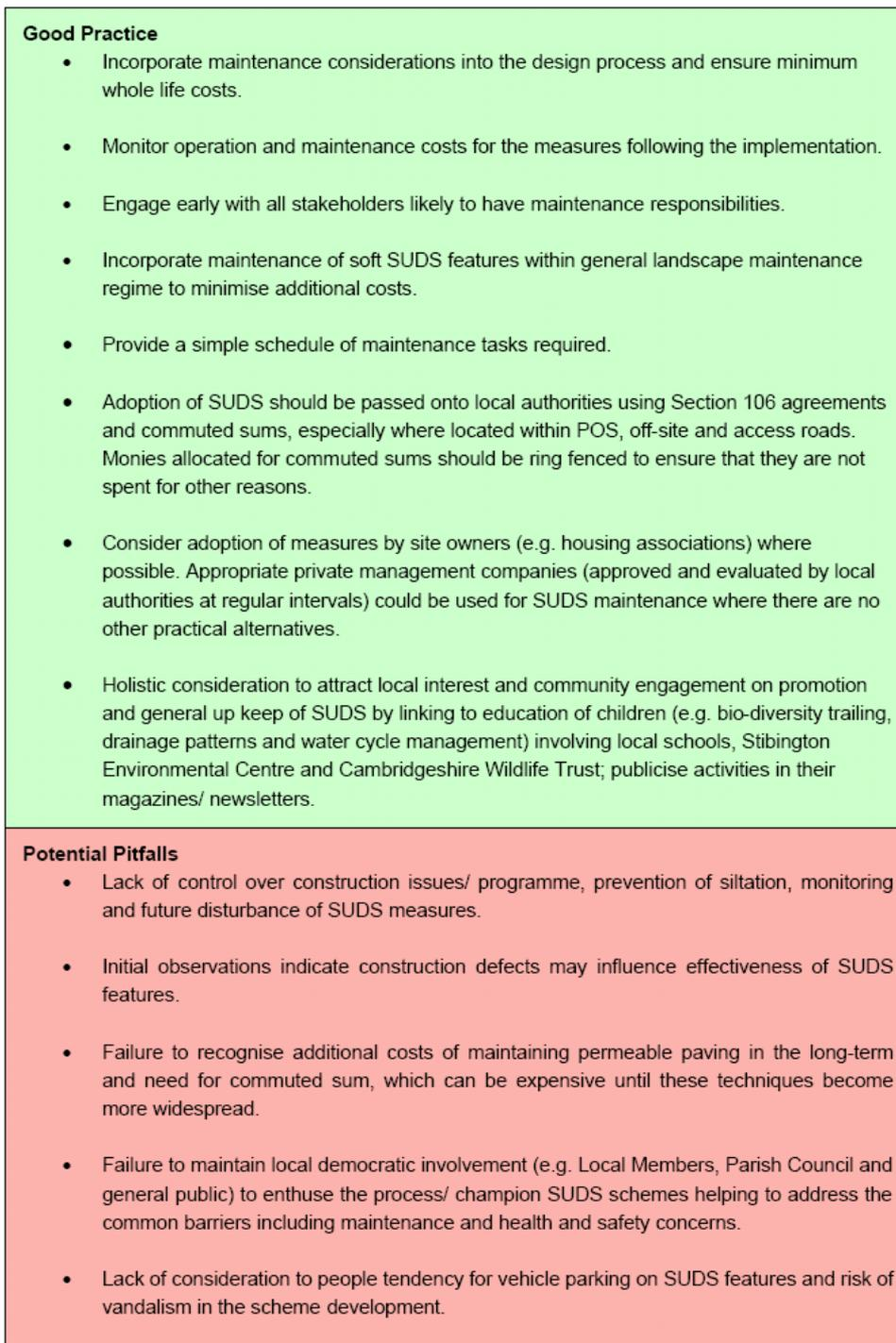
Figure 6-1 Guidance on management and operation of SuDS (Gunasakera et al 2006)
