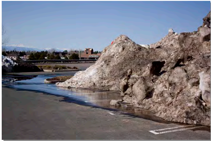
Photograph SIM-1. Snow storage locations should be clearly communicated to snow removal contractors and located where they can drain to stormwater BMPs or landscaped areas. Photo courtesy of WWE.
