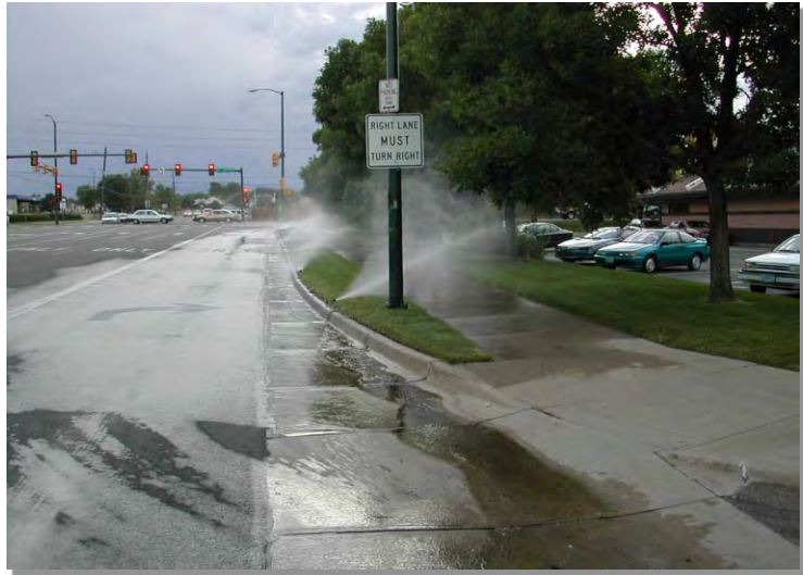
Photograph LM-1. Over-irrigation and overspray can wash fertilizers and lawn chemicals into the storm drain system. These flows can come together with storm runoff and cause nuisance flow conditions in stormwater BMPs. Photo courtesy of the City of Westminster.
