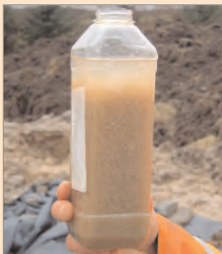
Water sample 15 seconds after adding the flocculant
