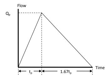
Figure 3-13 SCS (NRCS) triangular unit hydrograph (NRCS, 2007).
