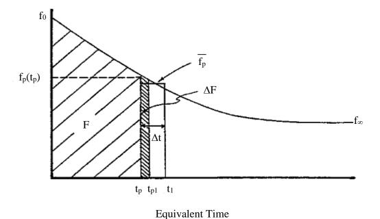
Figure 4-3 Cumulative infiltration F as the area under the Horton curve.
