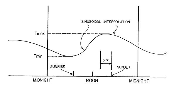
Figure 2-1 Sinusoidal interpolation of hourly temperatures.
