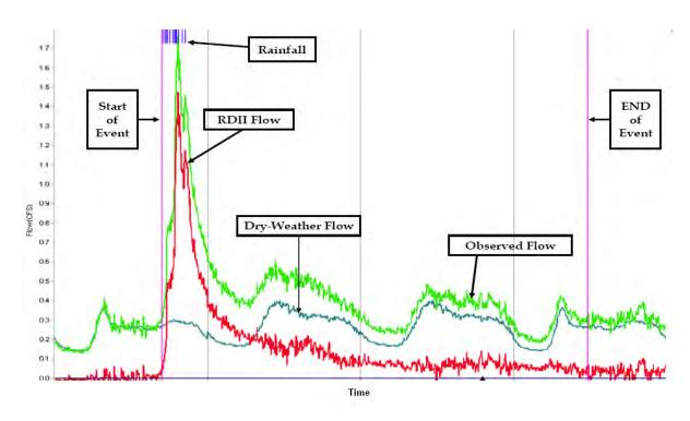
Figure 7-6 Extracting RDII flow from a continuous flow monitor (Vallabhaneni et al., 2007).
