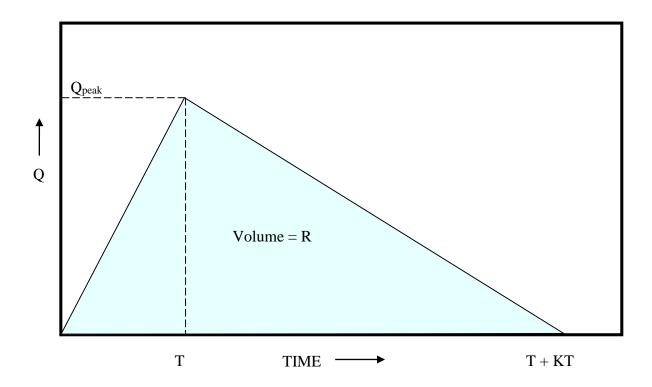
Figure 7-2 Example of an RDII triangular unit hydrograph.
