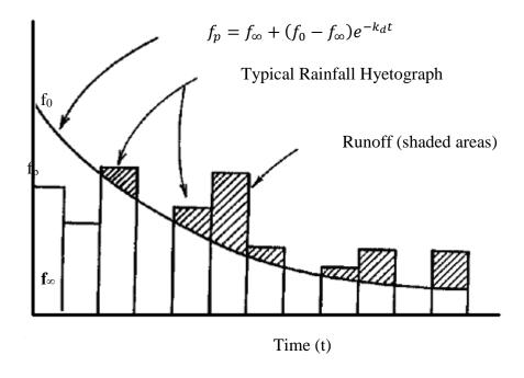
Figure 4-2 The Horton infiltration curve.
