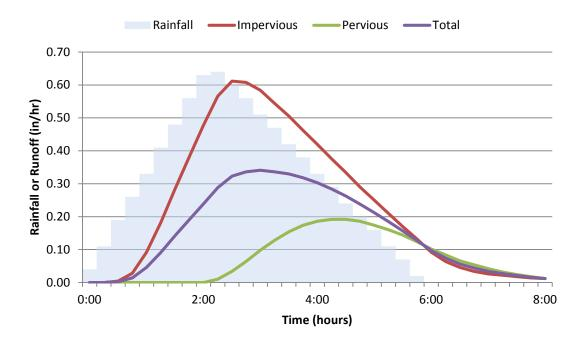
Figure 3-12 Runoff results for illustrative example.
