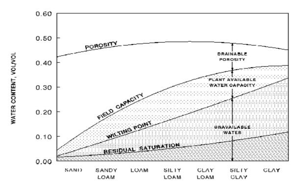
Figure 5-3 Relation between soil moisture limits and soil texture class (Schroeder et al., 1994).
