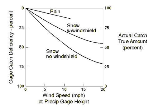
Figure 6-1 Typical gage catch deficiency correction (Anderson, 2006, p. 8).
