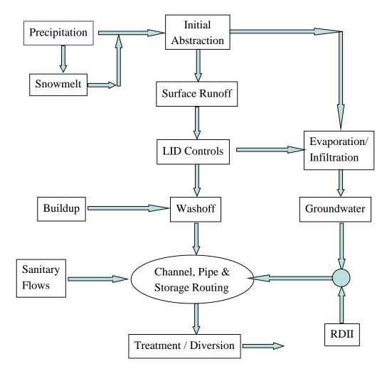
Figure 1-3 Processes modeled by SWMM.
