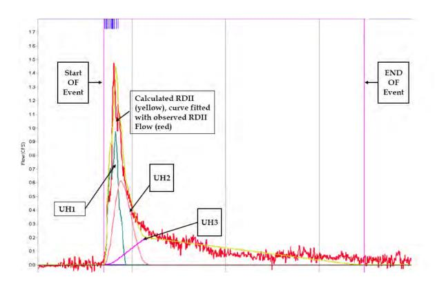
Figure 7-7 Fitting unit hydrographs to an RDII flow record (Vallabhaneni et al., 2007).
