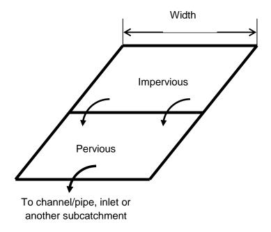
Figure 3-5 Re-routing of overland flow (Huber, 2001).
