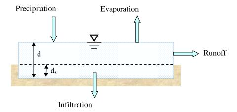
Figure 3-2 Nonlinear reservoir model of a subcatchment.
