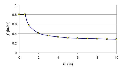
Figure 4-6 Illustration of infiltration capacity as function of cumulative infiltration for the Green-Ampt method.
