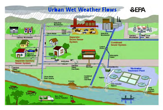
Figure 1-1 Elements of a typical urban drainage system.
