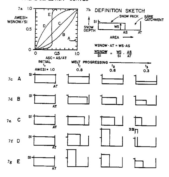
Figure 6-5 Effect of snow cover on areal depletion curves.
