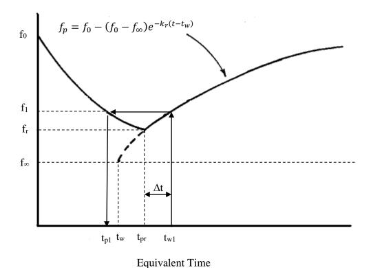
Figure 4-4 Regeneration (recovery) of infiltration capacity during dry time steps.
