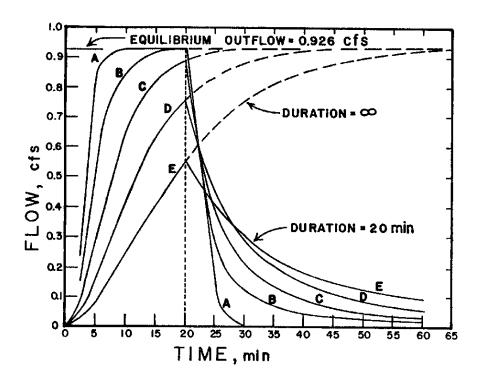
Figure 3-10 Subcatchment hydrographs for different shapes of Figure 3-9.
