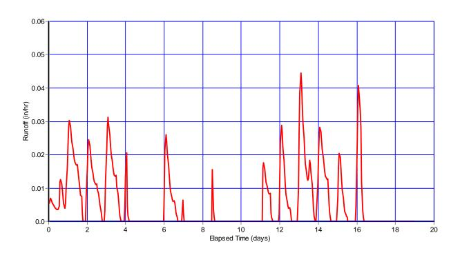
Figure 6-10 Runoff time series for illustrative snowmelt example.
