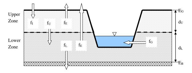
Figure 5-1 Definitional sketch of the two-zone groundwater model.
