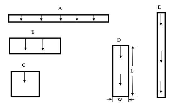
Figure 3-9 Rectangular subcatchments for illustration of shape and width effects.
