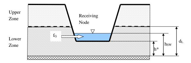
Figure 5-2 Heights used to compute lateral groundwater flow rate.
