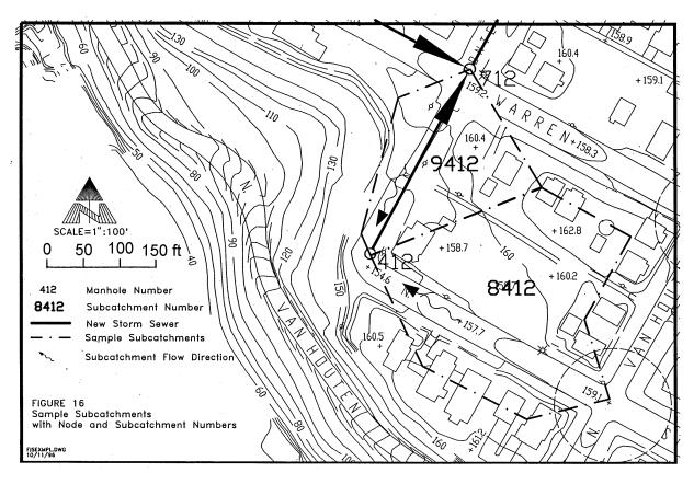
Figure 3-7 Detailed view of two Fisk B subcatchments (Portland BES, 1996).
