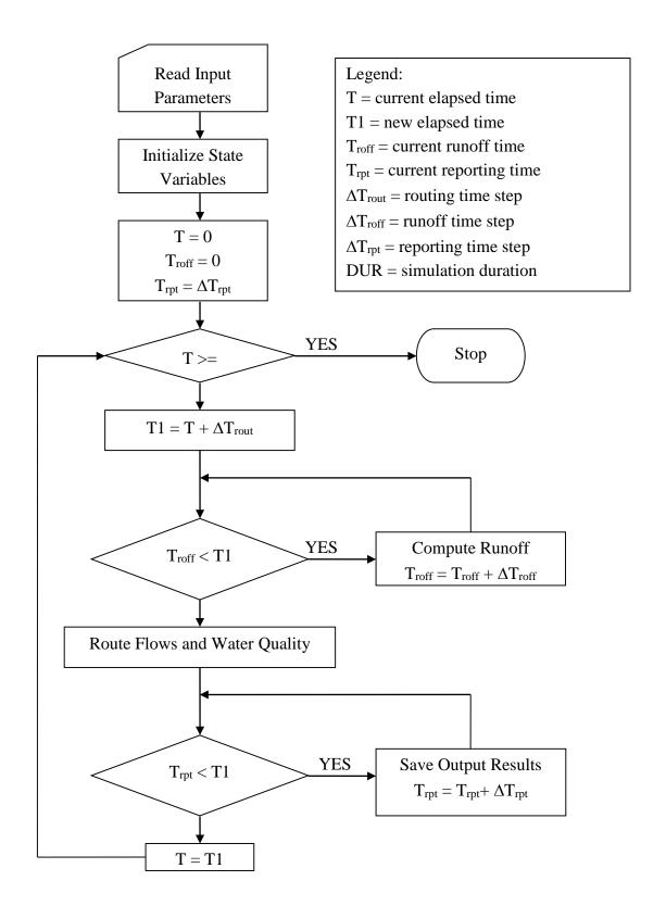
Figure 1-5 Flow chart of SWMM's simulation procedure.
