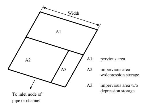
Figure 3-4 Idealized subcatchment partitioning for overland flow.
