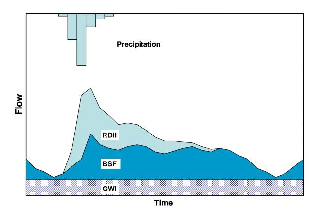
Figure 7-1 Components of wet-weather wastewater flow.
