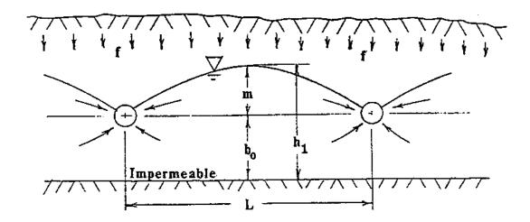
Figure 5-8 Definition sketch for Hooghoudt's method for flow to circular drains.
