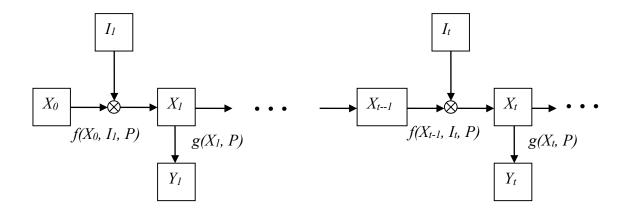
Figure 1-4 Block diagram of SWMM's state transition process.
