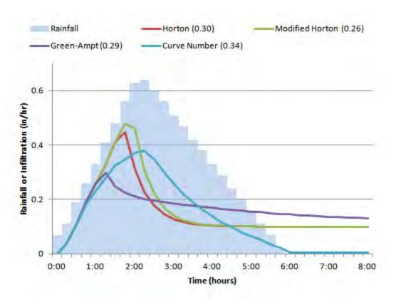
Figure 4-8 Infiltration rates produced by different methods for a 2-inch rainfall event. (Numbers in parentheses are the fraction of rainfall that becomes runoff.)
