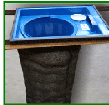
Catch basin insert incorporates a specialized filtration fabric and a mesh lining to remove various types of pollutants (Source: CleanwayUSA)
