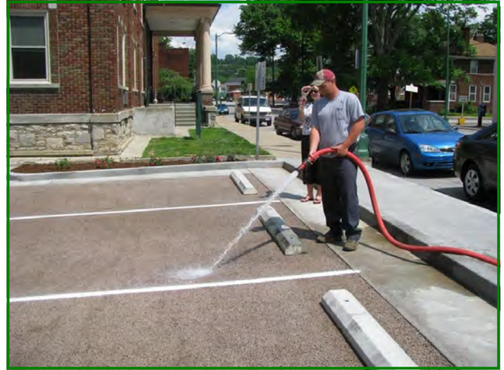
Test and observe infiltration on pervious pavements (Photo: Kentucky Concrete Pavement Association)
