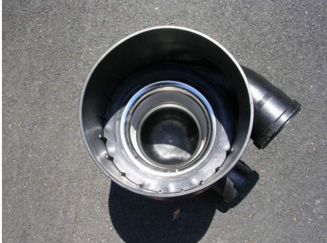
Figure S4.6. Interior of Vortex Filter
