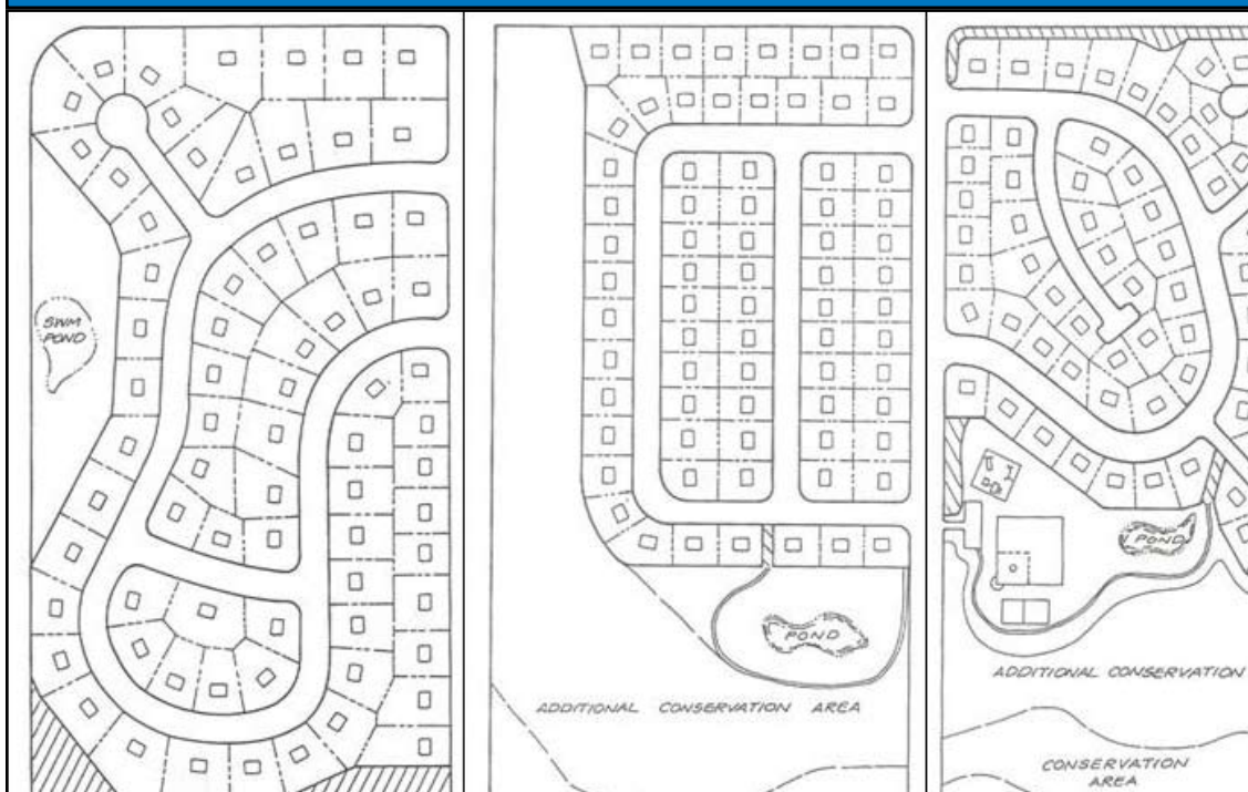
Figure 4.4 Conventional Subdivision (left) with 72 Lots, an Alternative Layout (center) Using Open Space Design with the Same Number of Lots, and Another Alternative Layout (right) Using Open Space Design with 66 Lots (Source Schueler, 1995)
