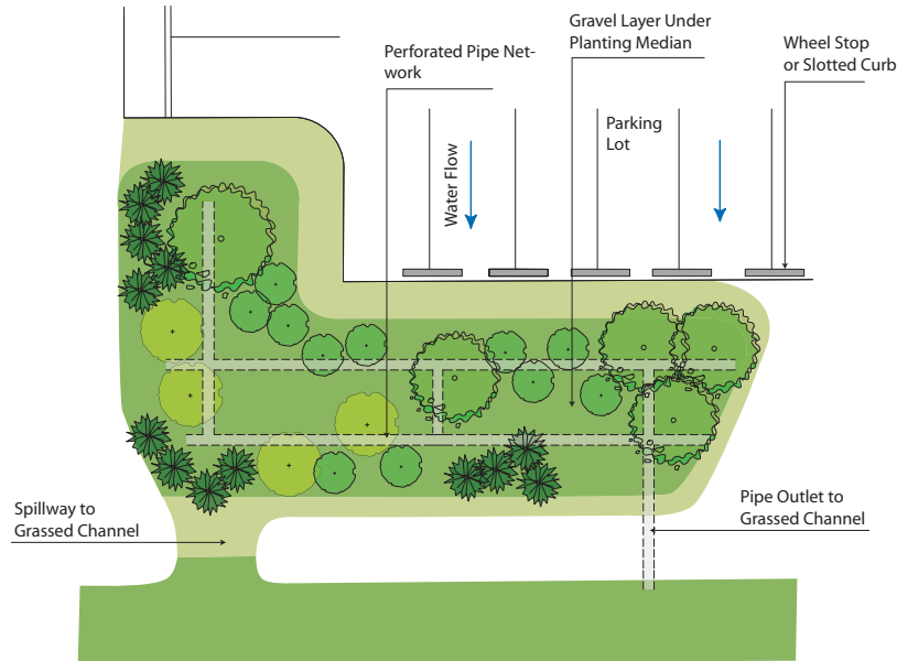
Raingarden example with underdrain
