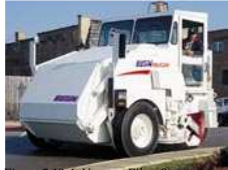
Figure 5.13-1 Vacuum Filter Street Sweeper
