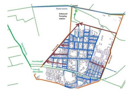
The "pumping station", raising water from the canal, was created as independent infrastructure in order to properly account for Energy and Emissions associated to the pumps' construction and set in place. The drainage surface of such infrastructure is anyway considered as null.
