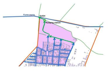
The pumping station is equipped with two pumps (with a design discharge of 500 l/sec each, whereof only one is working due the lack of an adequate connection to the electric grid) and is design for a return period of 30 years.
