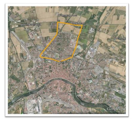
The selected area is part of Fiume Morto drainage system. The area is mainly served by a separate wastewater grid connected to a wastewater treatment facility (San Jacopo 40.000 PE) and partly by a combined network.
