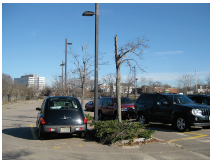
Figure 6-5 Example of Poorly Designed Parking Lot Landscaping.
