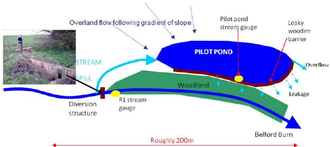
2. The spill point is created by lowering the riverbank to a predetermined flood level or by constructing a simple in-channel control structure.
