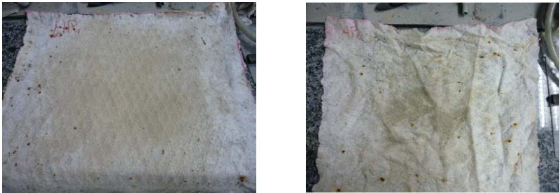
Figure 27. Detail of the sediments that infiltrated through the surface and the base layers and got trapped by the geotextile.
