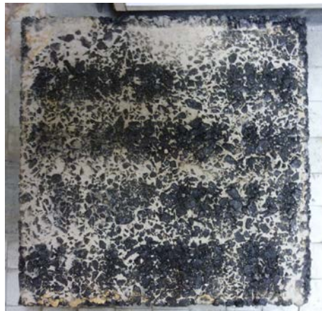
Figure 15. Scheme of the two main zones of study: clogged zone where the drops did not touch the surface and less clogged zone where the drops touched the surface and take away the sediments.
