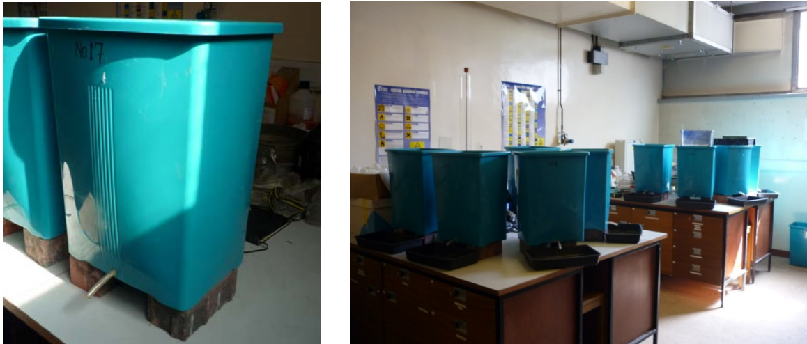
Figure 13. (Left) Hole with a pipe at the bottom of the bin to measure the volume of water infiltrated and (right) scheme of the 9 bins used to simulate the three sections of permeable pavements.
