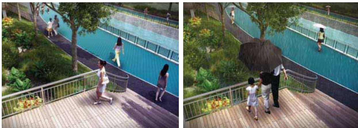
Figure 6.1.2 Bioretention basin during dry weather (left). During a rain event (right), stormwater is directed into the swale, reducing the velocity and volume of runoff into the drainage system.
