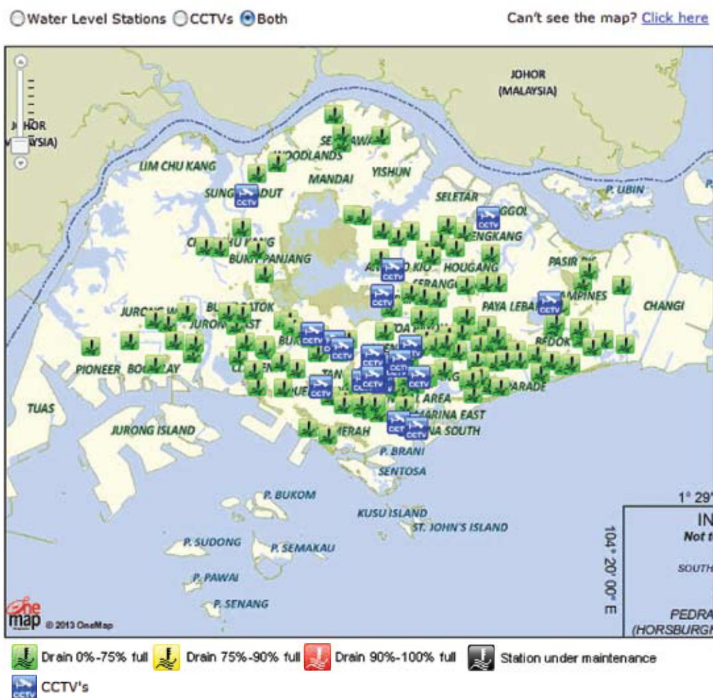
Figure 4.18 Location of water level sensors and CCTV's for flood monitoring in Singapore, available on the PUB website and MyWaters mobile app.
