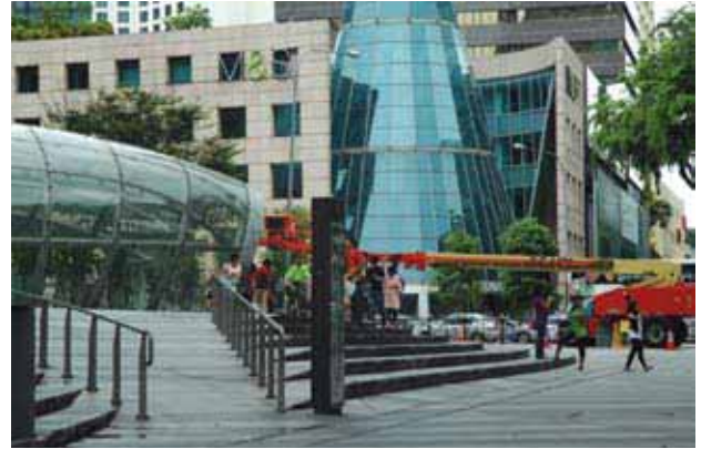
Figure 4.3 Steps and ramps are some of the options to achieve the minimum platform levels for developments with entrances to underground facilities.
