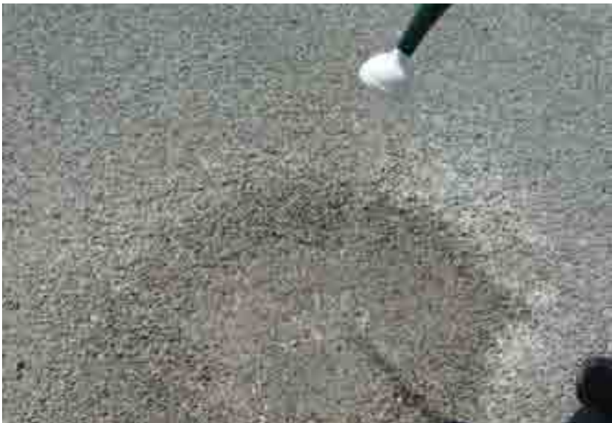
Porous concrete lets water permeate down to the subsurface soil
