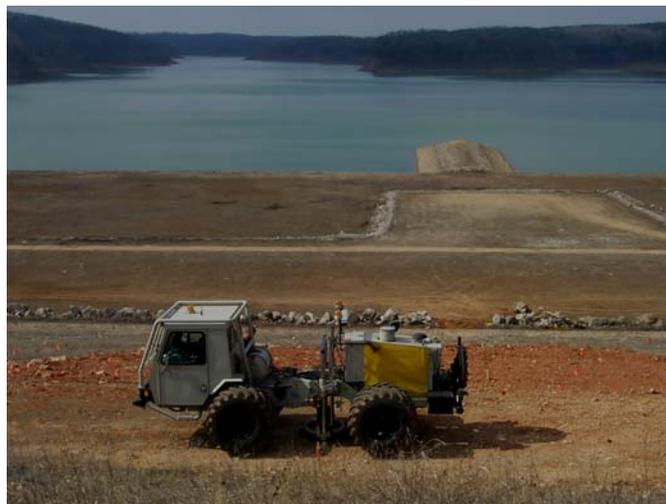
Figure 15. Mini-Vib seismic source for geophysical investigations Clearwater Dam (Source: Miller et al, SAGEEP 2004)
