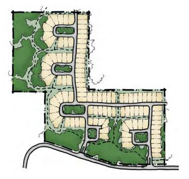
FIGURE 3.5 LOOP AND GRID HYBRID STREET NETWORK Loop and grid hybrid street network serving residential uses Source: AHBL, Inc. courtesy of Low Impact Development Technical Guidance Manual for Puget Sound (2012)
