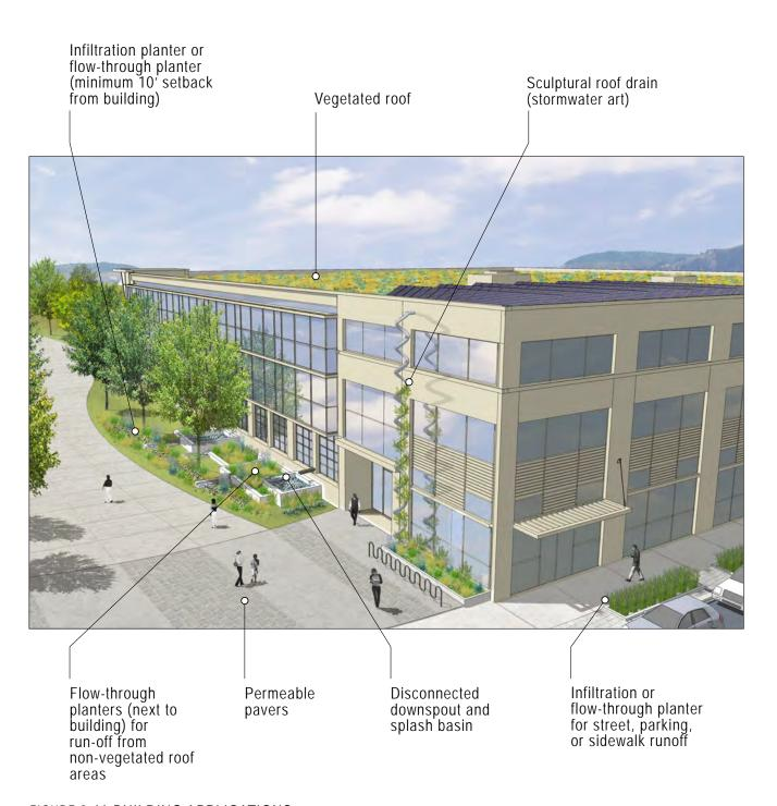
FIGURE **3.11 BUILDING APPLICATIONS** Source: CleanWater Services
